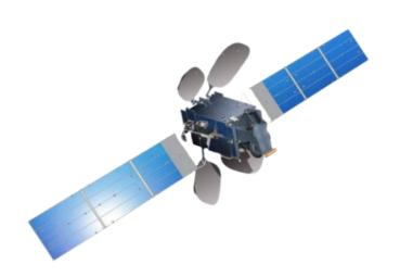
Manufacture SSL/MAXAR Launcher Ariane 5, Arianespace **Spacecraft Separated** Mass Contract 28 April 2014 mass 3500 Kg 150.5° E **Position** Age 15 Years **Above Equator** Launch 36 x 36 MHz **Transponder** Kurou Location 9 x 72 Mhx
